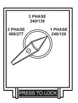
Figure 40. Voltage Selector Switch
